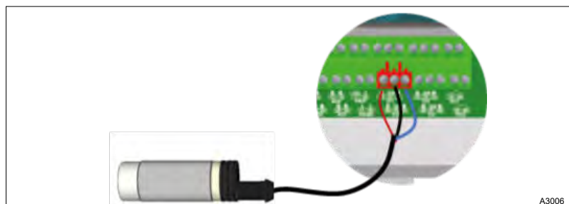
Fig. 22: Connection of a flow switch sensor to DI2
