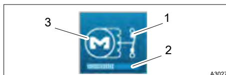
Fig. 40: Relay output in metering mode
