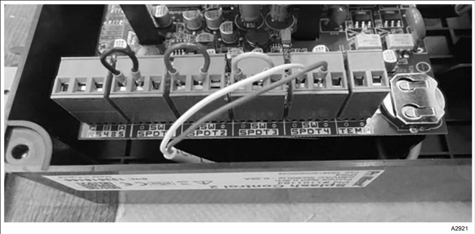
Fig. 10: Splash Control 2 with connected DGMA and bridges on the non-assigned terminals.
