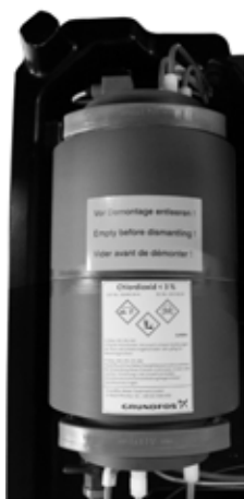
Fig. 39 Reaction tank with internal batch tank of OCD-162-10
