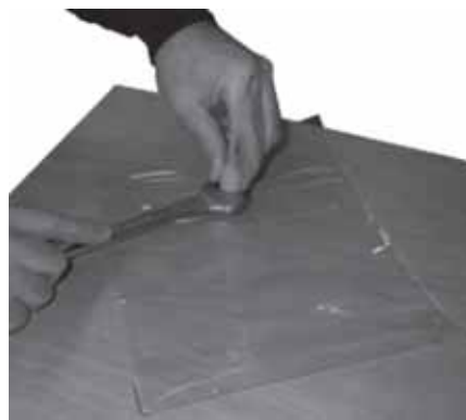
Fig. 46 Replacing the volume compensation bag
