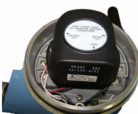
Figure 2-5. Installing the Power Module
